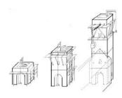
"Putlog holes" used to support scaffolding can still be seen on each side of the tower. Stones (and stonemasons as well) were probably winched up on a wheel wedged inside the tower.
